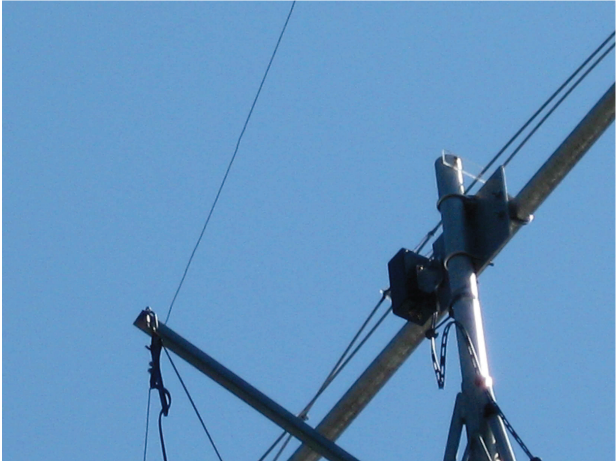
Figure 6. A closer view of the middle of the array. The black object just to the left of the mast-boom junction is the box containing the 1:2 balanced transformer. This view also shows more clearly the twisted phasing line made from \frac{1}{4} " aluminum rod. The Plexiglas spacer at the top of the mast holds the center of the phasing line about 8" above the boom.
